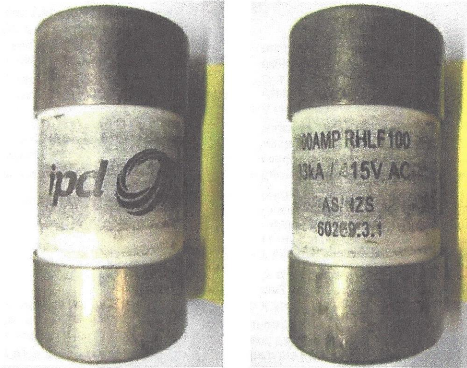
An ipd brand of HRC fuse and example markings
